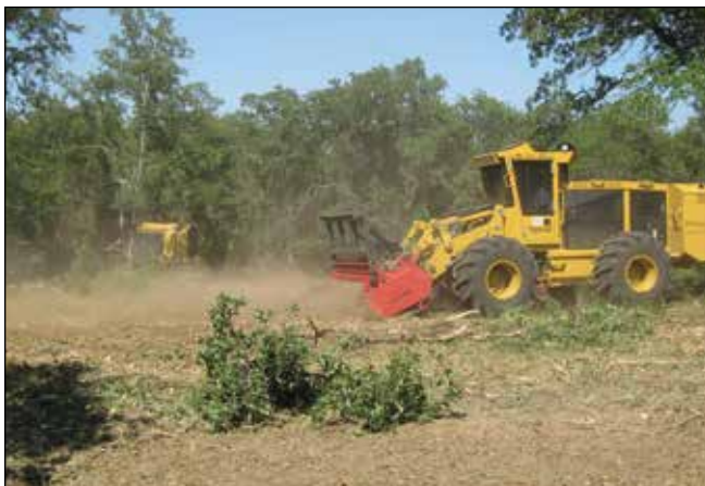
Figure 17. Mulchers and other heavy equipment can be effective for reducing canopy coverage, allowing more beneficial and diverse understory vegetation to grow. Photo by National Wild Turkey Federation.
