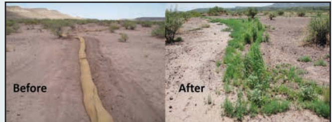
Figure 3. Restoration experiment of a sodic soil using cotton bur burlap wattles. Photo provided by Bonnie Warnock, Sul Ross University.
