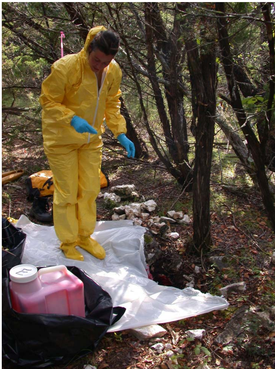
Figure 6. Injecting eosin dye at site WF94
