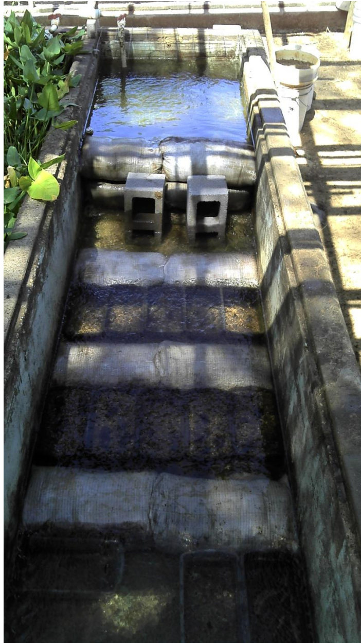
Figure 1. Photo of raceway at LAERF. Water flows from top to bottom of photo. Mussels are held in sediment filled plastic shoe boxes behind sandbags that mimic riffles. Inflowing water first enters a settling pool to remove suspended solids and increase dissolved oxygen concentration as it spills over the barrier wall.
