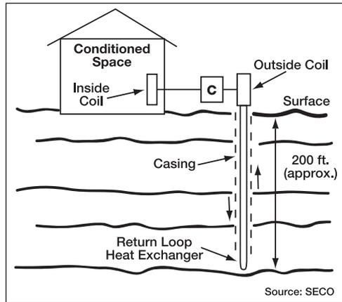
Although “geothermal heat” may make us think of geysers and red-hot lava, the Pond Center’s classroom and lab are heated and cooled by a “ground-coupled geothermal” system. A conventional air conditioner extracts heat from a building and transfers the heat to the outside air through the condensing unit. The geothermal system works by transferring the building’s heat to the 74°F ground rather than Houston’s 94°F summertime air— a 20 degree difference!
