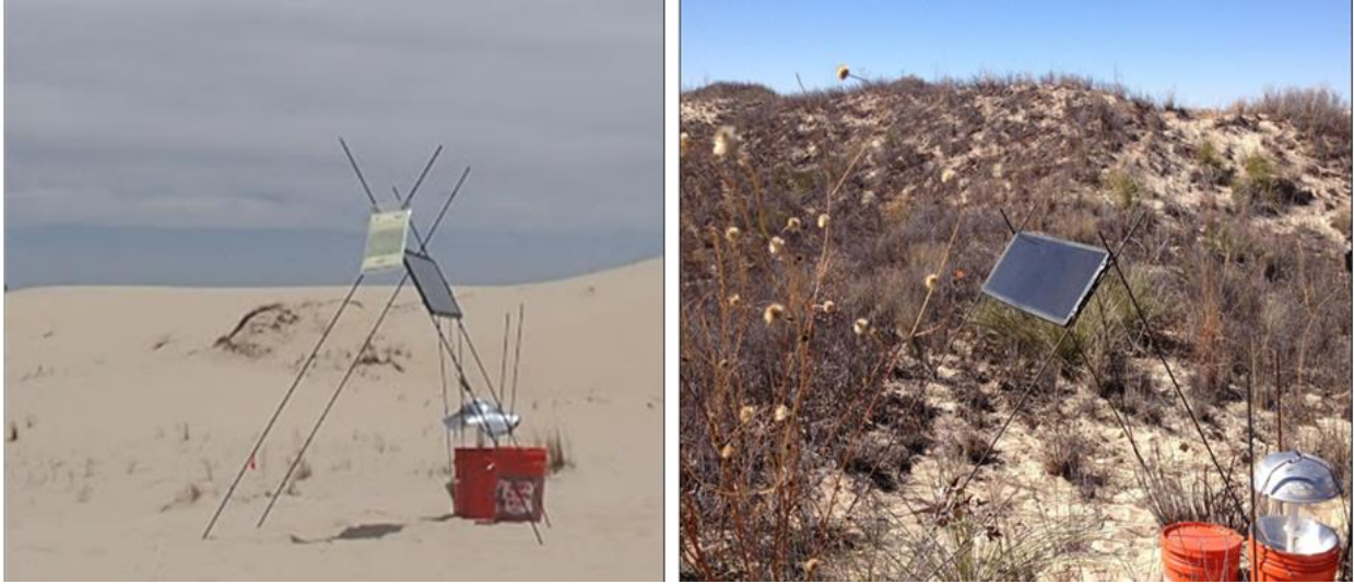
Figure 13. Solar-powered UV bucket light trap. These traps in addition to Townes traps and pitfall traps were established at each of the seven trapping stations (A-G) shown in Figure 12.
