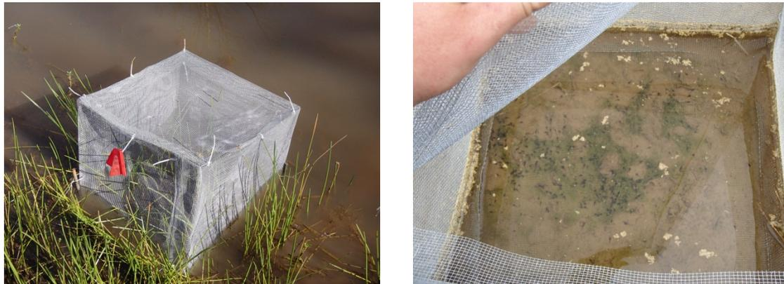
Figure 2. Egg enclosures used to reduce predation on released eggs and tadpoles. These are 1 x 1 m<sup>2</sup> enclosures built using 1/8 in hardware cloth.
