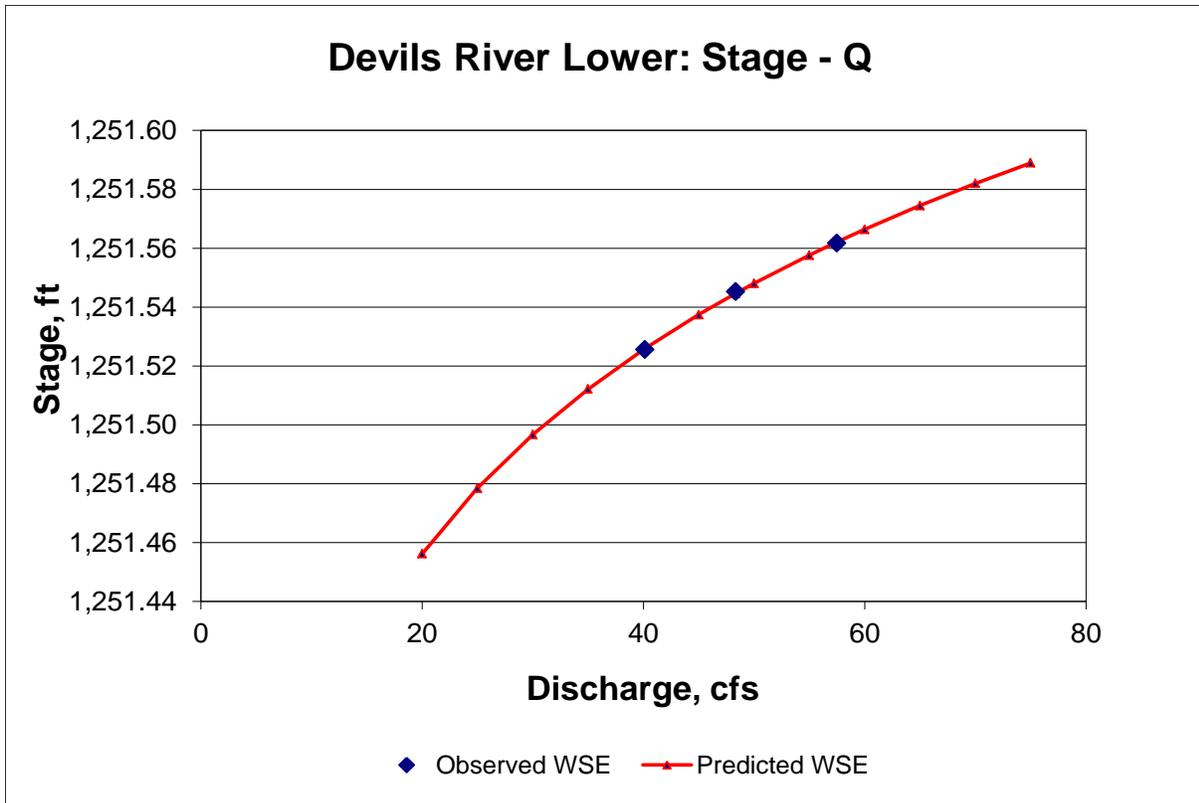
Figure A2. Stage (ft msl) versus discharge (cfs) relationship at the Devils River Lower site.
