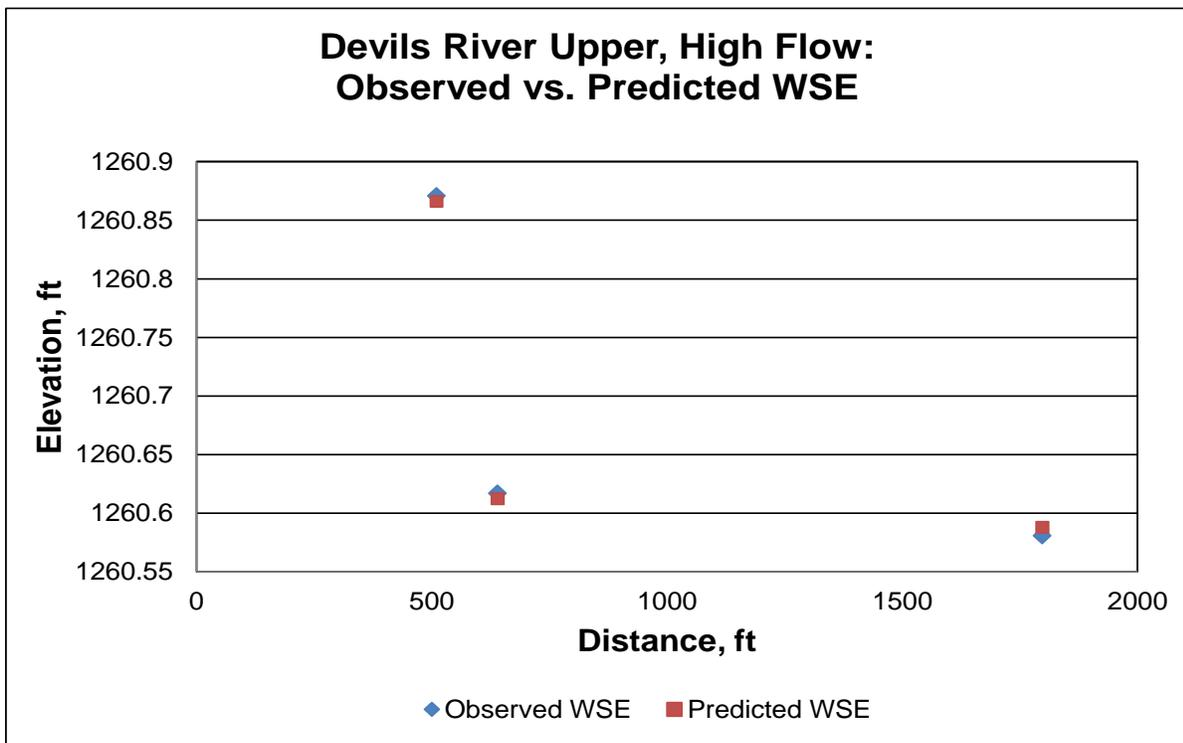
Figure A3. Comparison between observed and predicted water surface elevations (ft msl) at Devils River Upper site at high flow (February).
