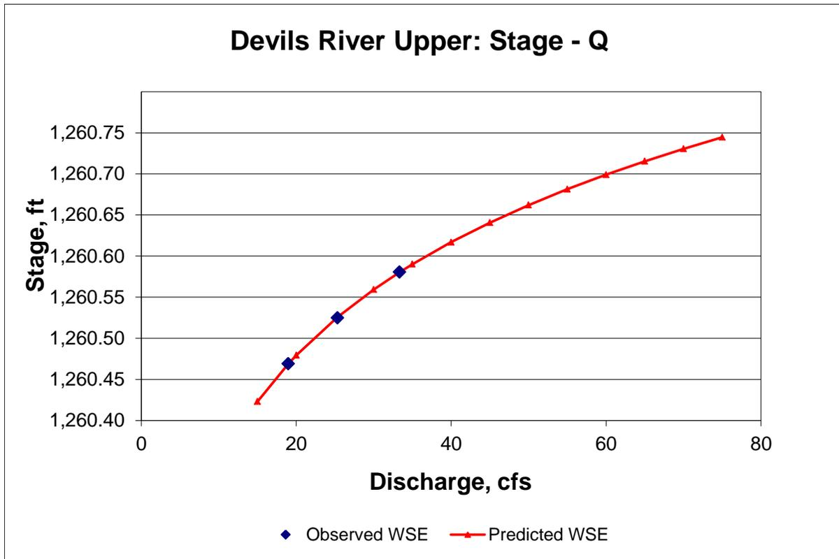
Figure A1. Stage (ft msl) versus discharge (cfs) relationship at the Devils River Upper site.
