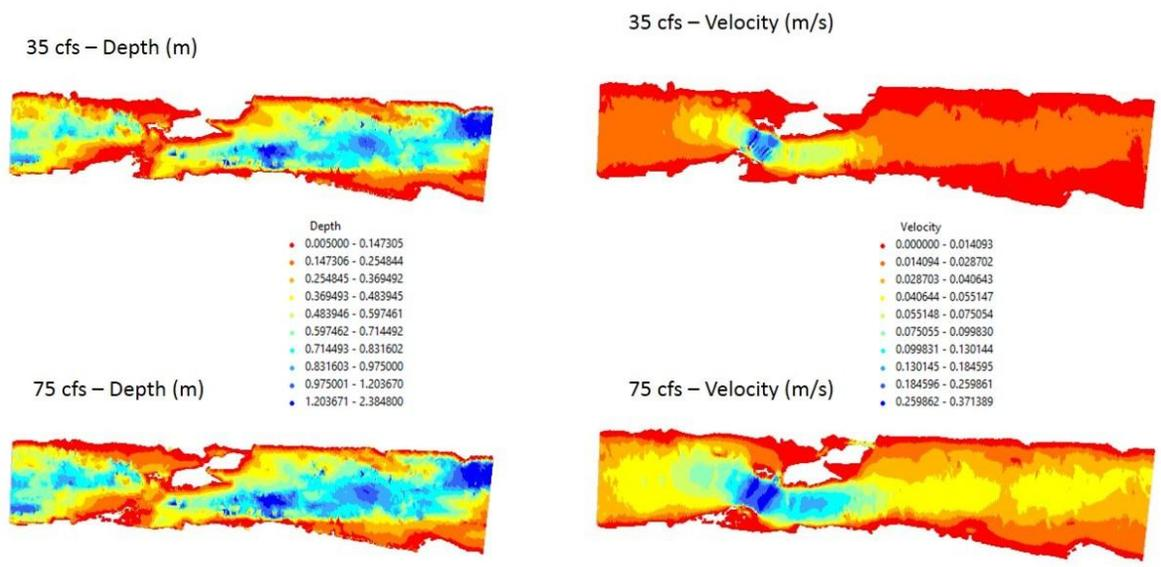
Figure 10. Depth and velocity contours at 35 and 75 cfs in the Devils River Upper site.
