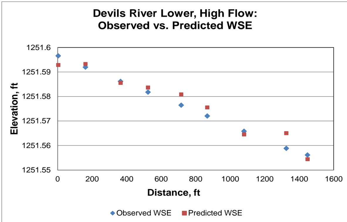
Figure A6. Comparison between observed and predicted water surface elevations (ft msl) at Devils River Lower site at high flow (February).
