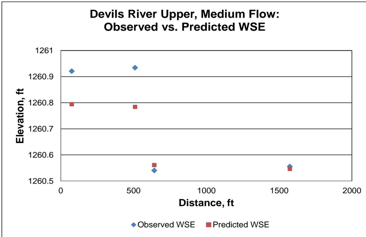
Figure A4. Comparison between observed and predicted water surface elevations (ft msl) at Devils River Upper site at medium flow (April).
