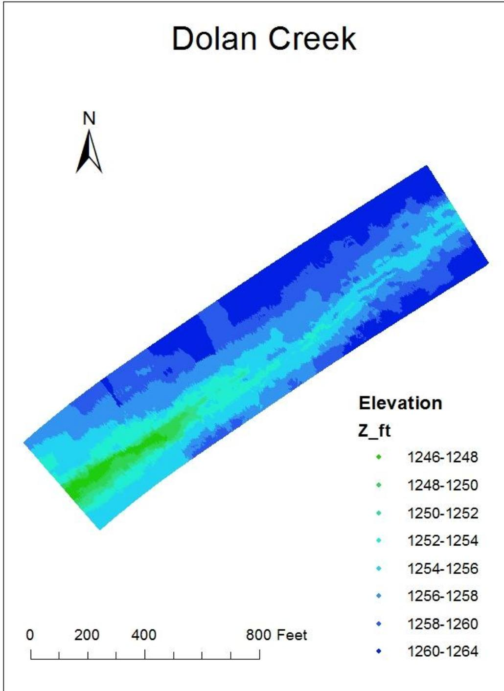
Figure 7. Computational mesh used in hydraulic modeling for Dolan Creek. It is 1668.8 ft long and 393.7 ft wide with a 1.5 x 1.5 ft cell size. The upstream boundary of the site is at the top of the figure. Elevation (Z) is feet above mean sea level.
