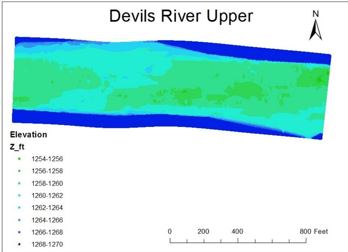
Figure 5. Computational mesh used in hydraulic and subsequent habitat modeling for Devils River Upper site. The mesh is 1830.8 ft long and 492.1 ft wide with a 2 x 2 ft cell size. The upstream boundary of the site is to the left. Elevation (Z) is feet above mean sea level.
