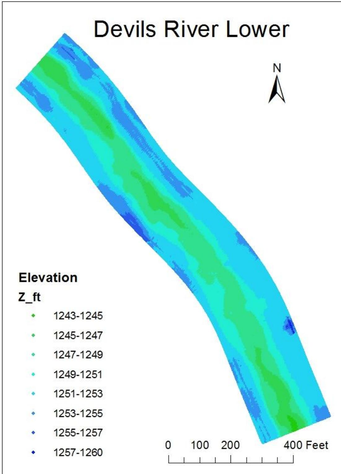
Figure 6. Computational mesh used in hydraulic and subsequent habitat modeling for Devils River Lower site. The mesh is 1454.3 ft long and 229.7 ft wide with a 1.6 x 1.6 ft cell size. The upstream boundary of the site is at the top of the figure. Elevation (Z) is feet above mean sea level.
