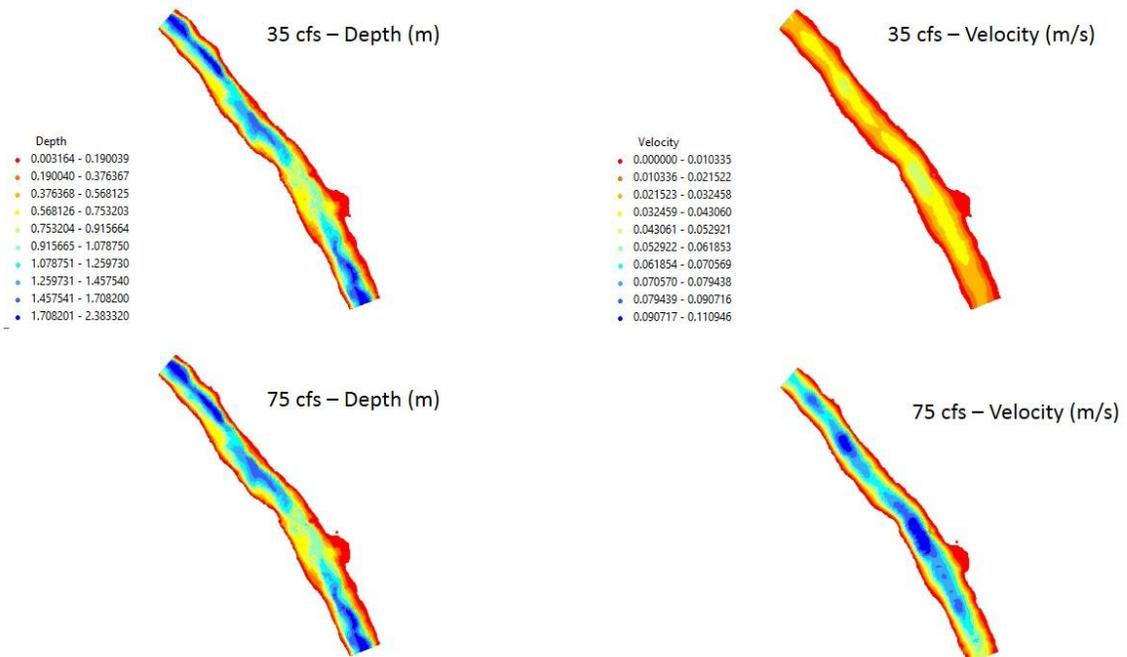
Figure 12. Depth and velocity contours at 35 and 75 cfs in the Devils River Lower site.
