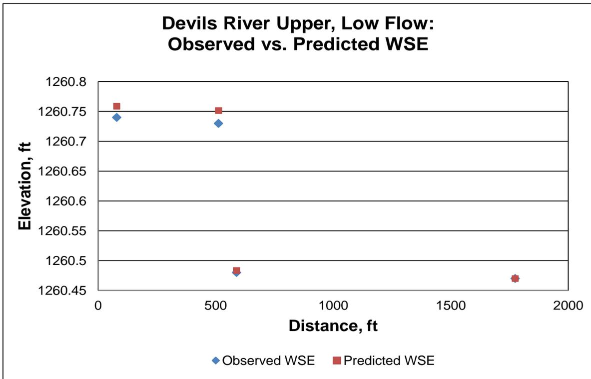
Figure A5. Comparison between observed and predicted water surface elevations (ft msl) at Devils River Upper site at low flow (September).
