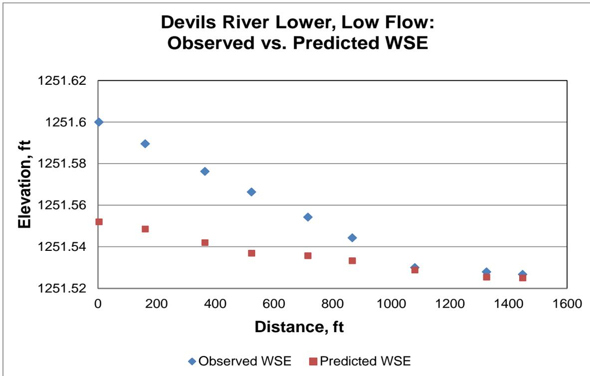
Figure A8. Comparison between observed and predicted water surface elevations (ft msl) at Devils River Lower site at low flow (September).
