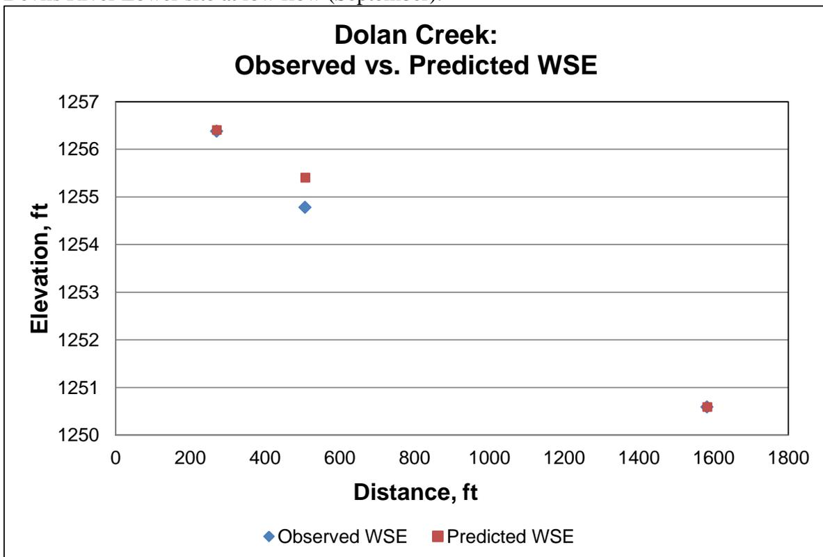
Figure A9. Comparison between observed and predicted water surface elevations at Dolan Creek at low flow (September).
