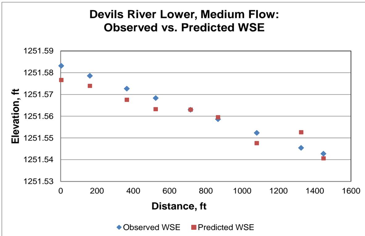
Figure A7. Comparison between observed and predicted water surface elevations (ft msl) at Devils River Lower site at medium flow (April).
