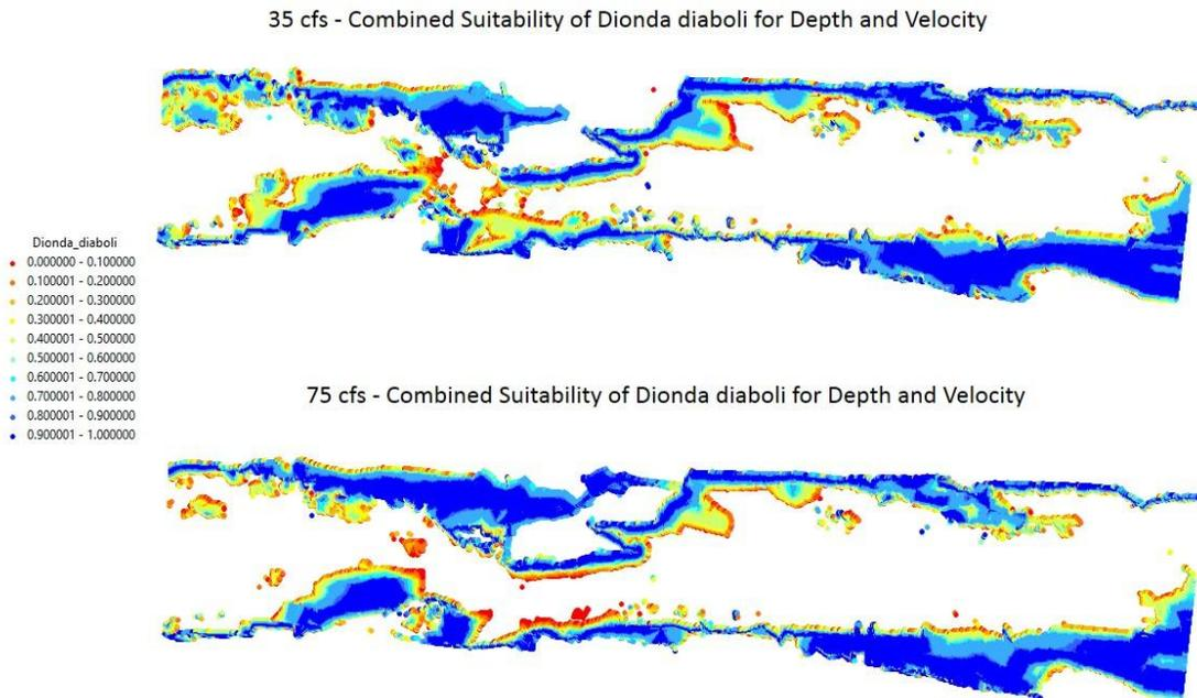
Figure 11. Comparison of combined depth and velocity suitability for Devils River Minnow within the Devils River Upper site at 35 and 75 cfs.
