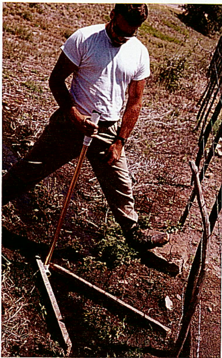
ABOVE: Matt Uliana is using the flowmeter in a field constructed flume to measure discharge at Catfish Springs
