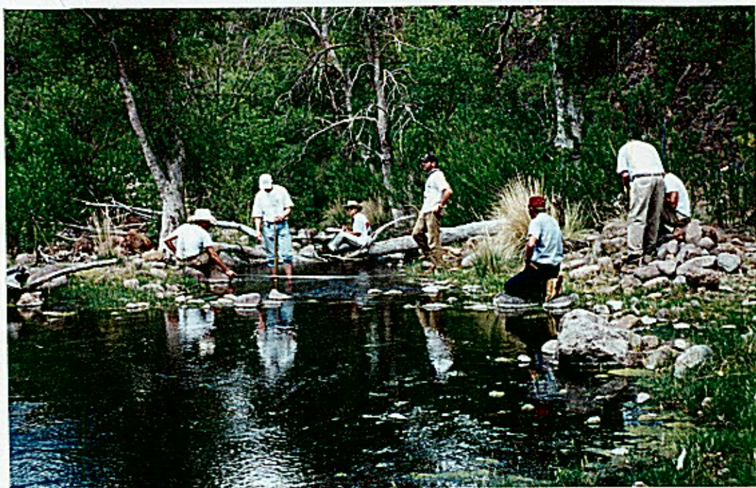
BELOW: Team members gauging the streamflow and discharge from a spring in the upper Big Aguja Canyon.
