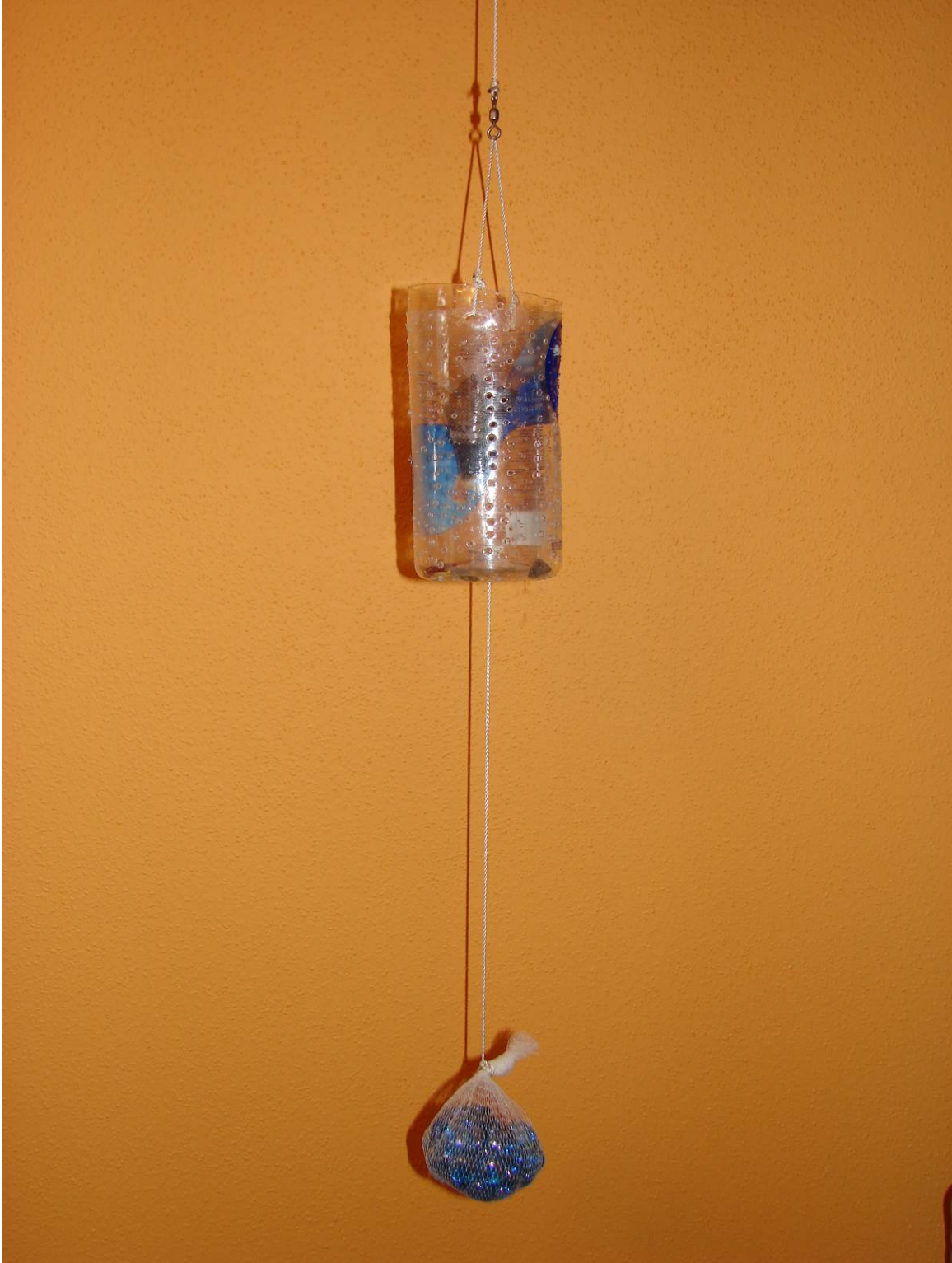
Figure 5. Bottle trap designed for open hole well sampling. This design has proven highly effective for sampling wells up to 300 feet deep.
