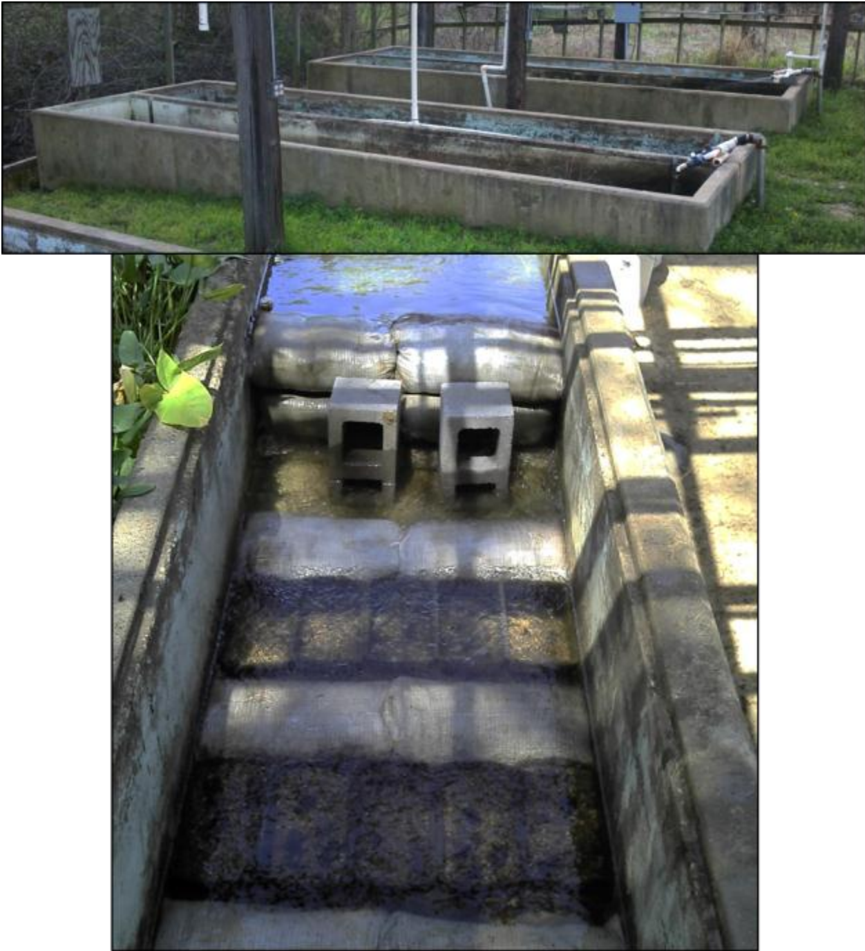
Figure 4. Outdoor raceways at LAERF modified to hold mussels in an artificial riffle.
