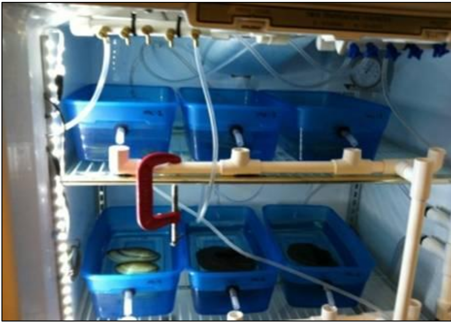
Figure 5. Refrigerated broodstock chamber with recirculating water filtration system.
