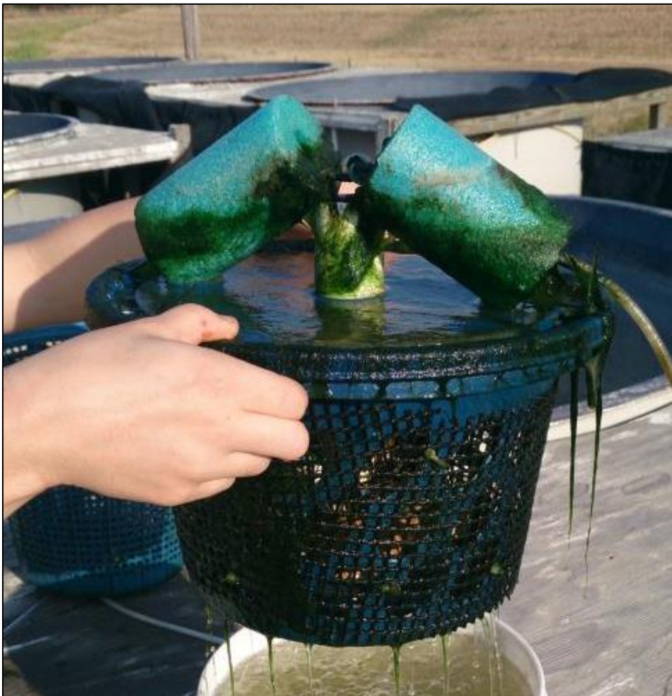
Figure 13. A floating mussel basket with air lift used in the 6000L mesocosm tanks.
