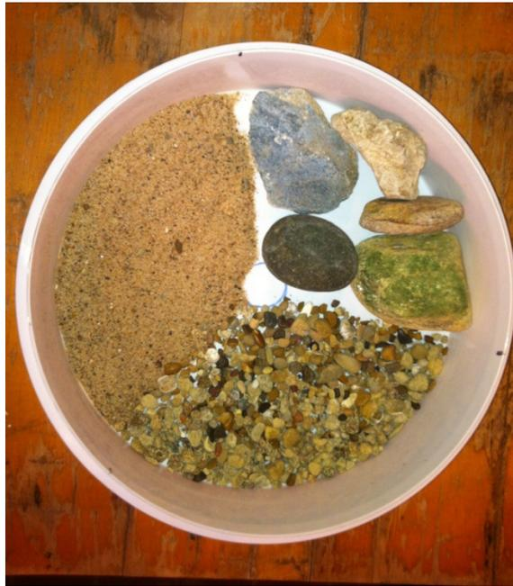
Figure 6.1--Chamber used in experimental trials, separated into three equally sized sections, with the three substrates, sand, gravel, and cobble.
