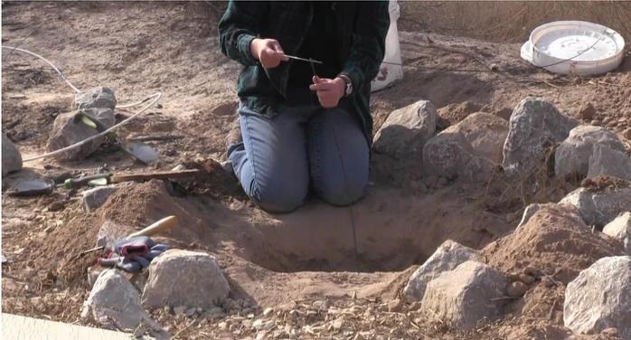
Attaching laundry brush segment of fish tape to the section of fish tape being pushed out the burrow to the entrance.
