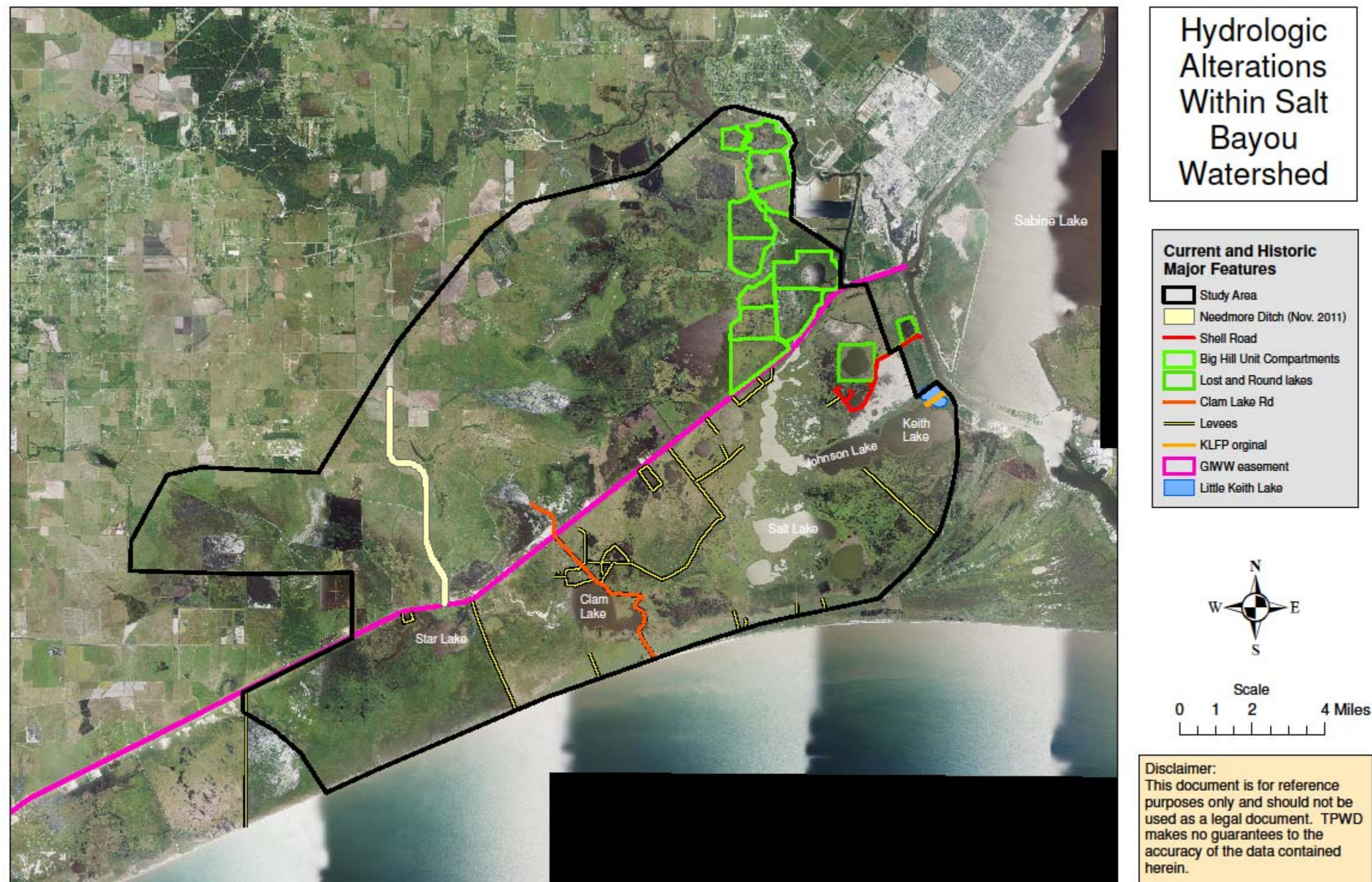
Figure 4. Major man-made structures that have resulted in significant hydrologic alterations.
