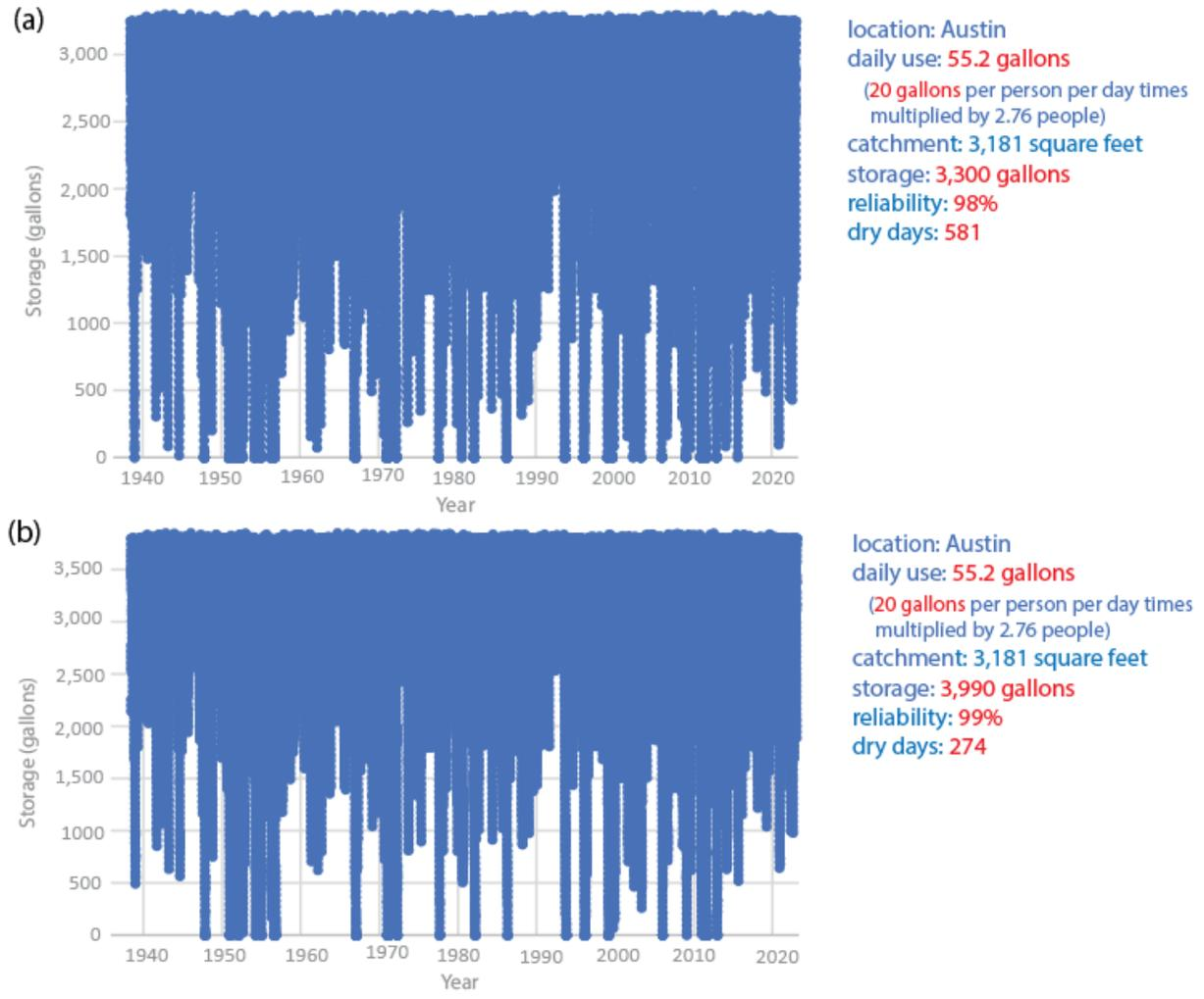
Figure 9: Storage performance and reliability for a couple rainwater systems in Austin.
