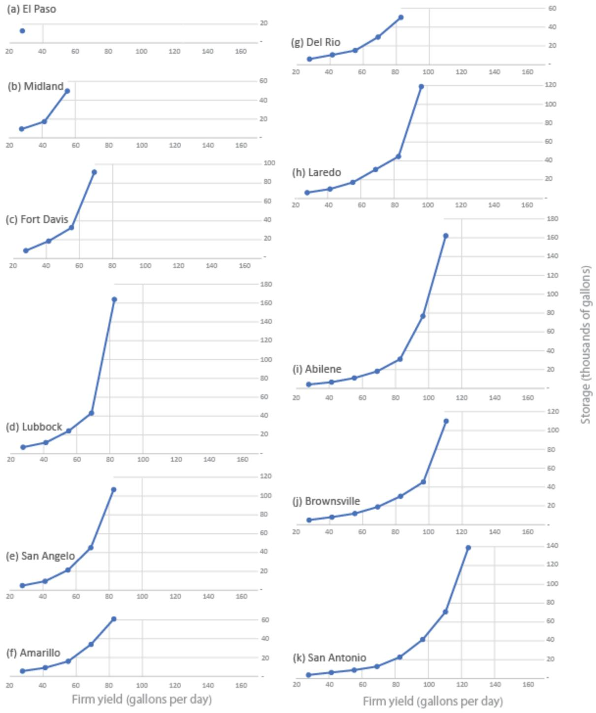
**Figure 2:** Storage required to achieve a range of firm yields for a catchment of 3181 square feet for a variety of Texas cities. I organized these graphs from least amenable to rainwater harvesting to most amenable. Note that each graph is on the same horizontal and vertical scale to allow direct comparison between plots. Also note that the plots end at the maximum achievable firm yield (for the use levels investigated).
