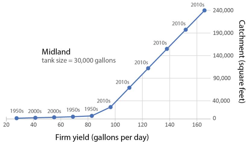
**Figure 7:** Example of increasing catchment area with increasing firm yield (use) for Midland including the decade the storage reaches a minimum (the decade of the end of the drought defining the firm yield).
