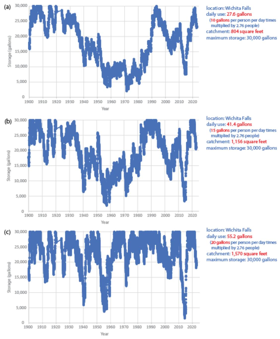
Figure 8: Storage performance for three demand/firm use scenarios with a set storage volume for Wichita Falls.
