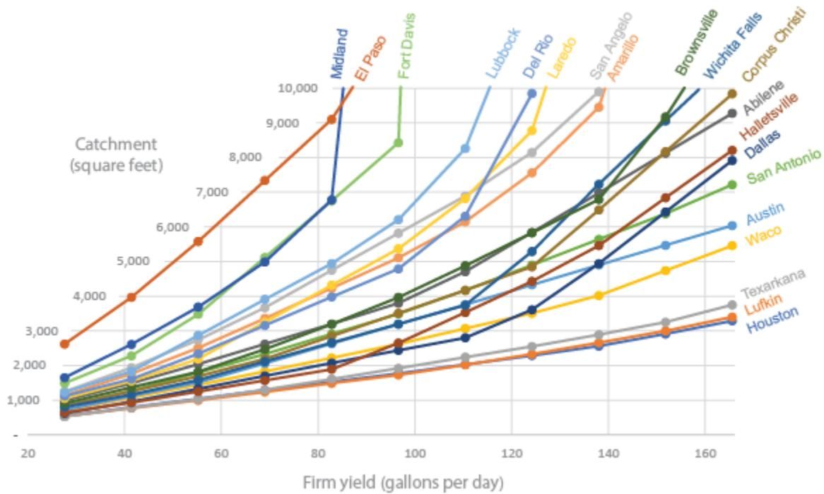
**Figure 6:** Catchment required to achieve a range of firm yields for storage of 30,000 gallons for a variety of Texas cities with storage capped at 50,000 gallons.
