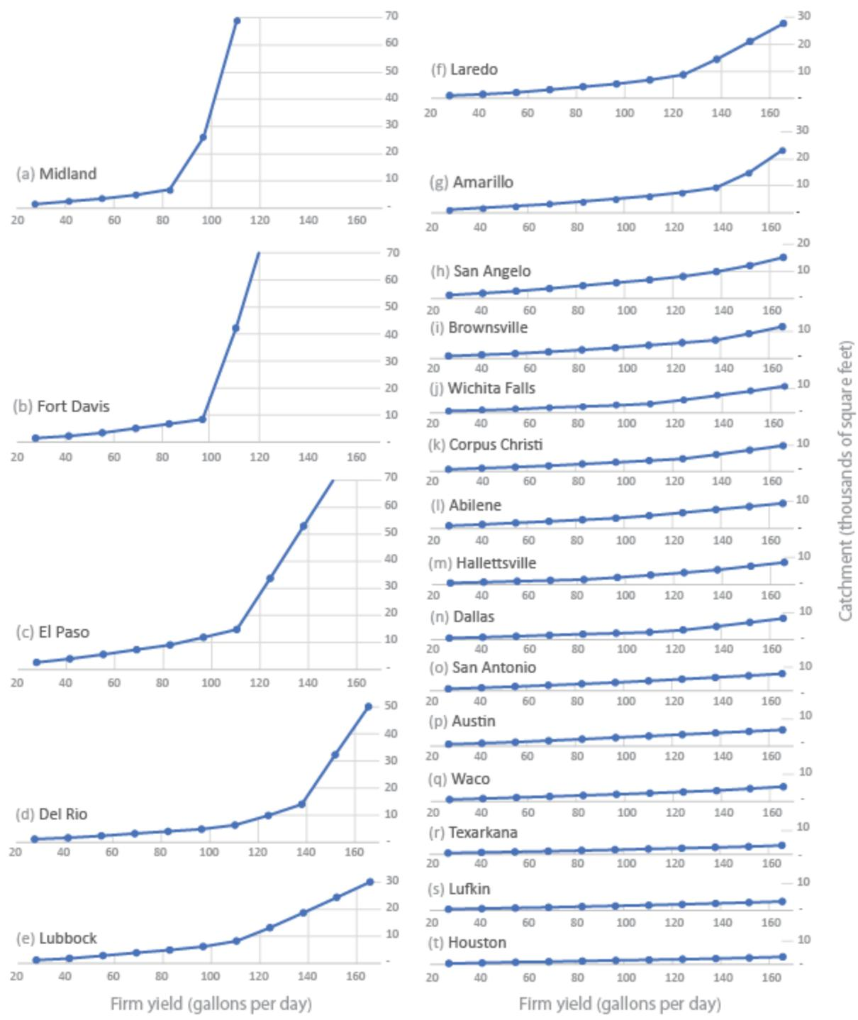
**Figure 5:** Catchment required to achieve a range of firm yields for a storage of 30,000 gallons for a variety of Texas cities. I organized these graphs from least amenable to rainwater harvesting to most amenable. Note that each graph is on the same horizontal and vertical scale to allow direct comparison between plots.
