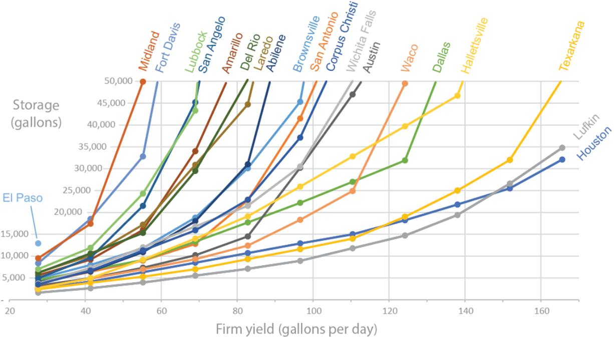
**Figure 3:** Storage required to achieve a range of firm yields for a catchment of 3181 square feet for a variety of Texas cities with storage capped at 50,000 gallons.
