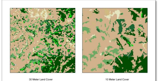
Figure 5. Illustration of the increase in spatial resolution from 30 meter pixels to 10 meter pixels. Image objects were generated from the first principle component of a NAIP image county mosaic that had been re-sampled to 10 meters.
