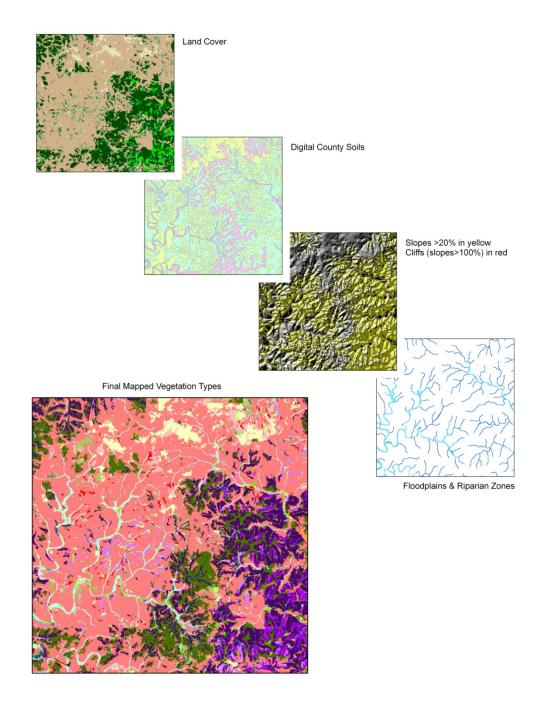
Figure 6. Example of data layers developed and used to map ecological systems, subsystems, and invasive types.
