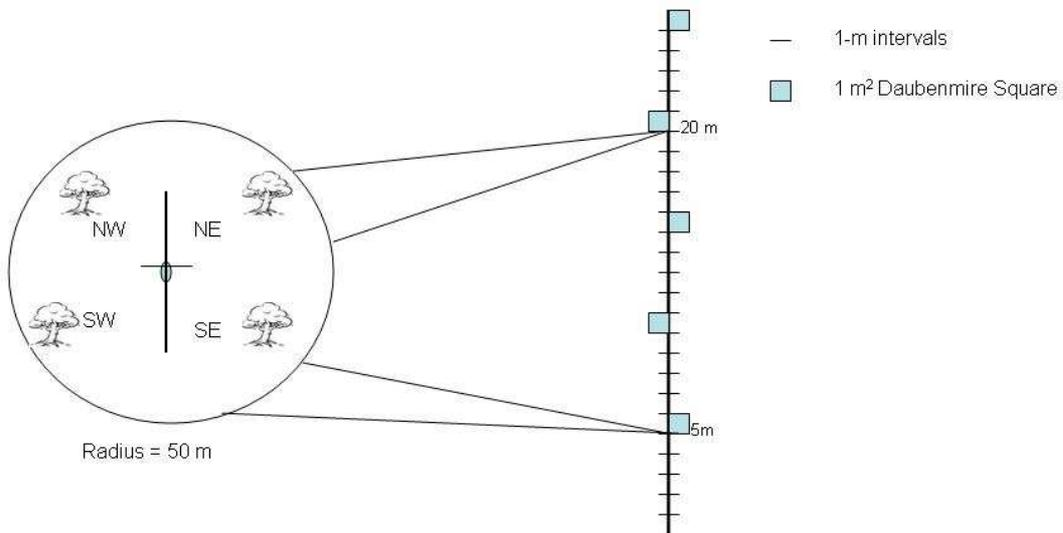
Figure 5. Plot arrangement used for vegetation surveys. The transect line is 25-m long, marked at 1-m intervals for line-intercept sampling. Herbaceous ground cover in a 1-m<sup>2</sup> square quadrat was measured at 5-m increments along the transect. At 5-m and 20 m, overstory vegetation was estimated using the point-centered-quarter method.
