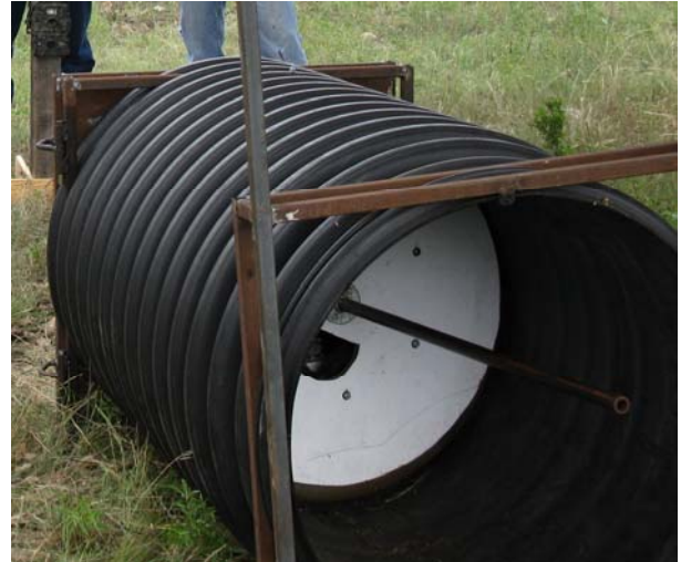
Figure 2. Trap door side of the Trap ‘N’ Gas with immobilizing plunger in place.
