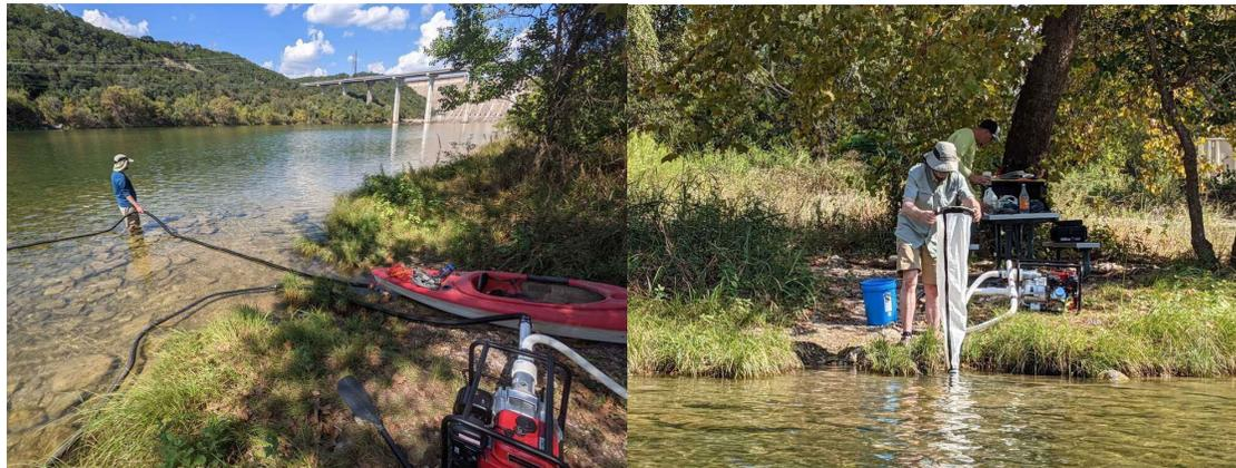
*Figure 2: These images are from below Mansfield Dam, 2021-09-18. In the left image, the kayak, water pump (foreground), and tubing are visible. On the right, the mesh net for sample collection (used for pump water) is visible.*
