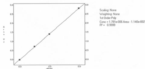
Fig. 1. Standard curve data for nitrate+nitrite analysis using Quikchem method 31-107-04-1-A.
