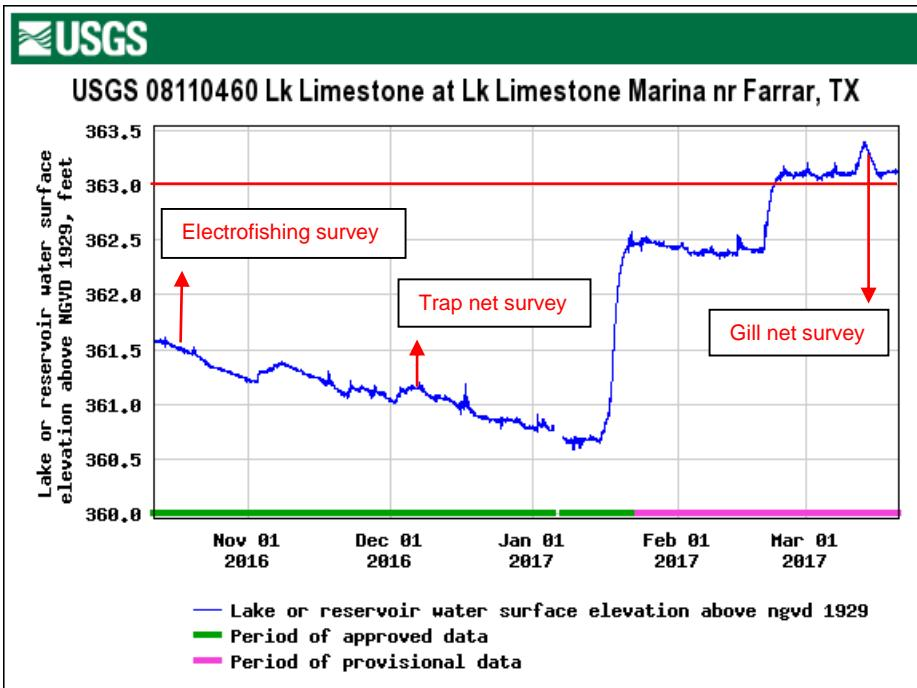
Figure 1b. Daily mean water levels for Limestone Reservoir for the 2016/2017 sampling season. Red arrows designate approximate days for electrofishing (October 12, 2016), trap net (December 6, 2016) and gill net (March 20, 2017) surveys. Conservation pool level (red line; no arrows) is 363 feet above MSL. Figure from the USGS website.
