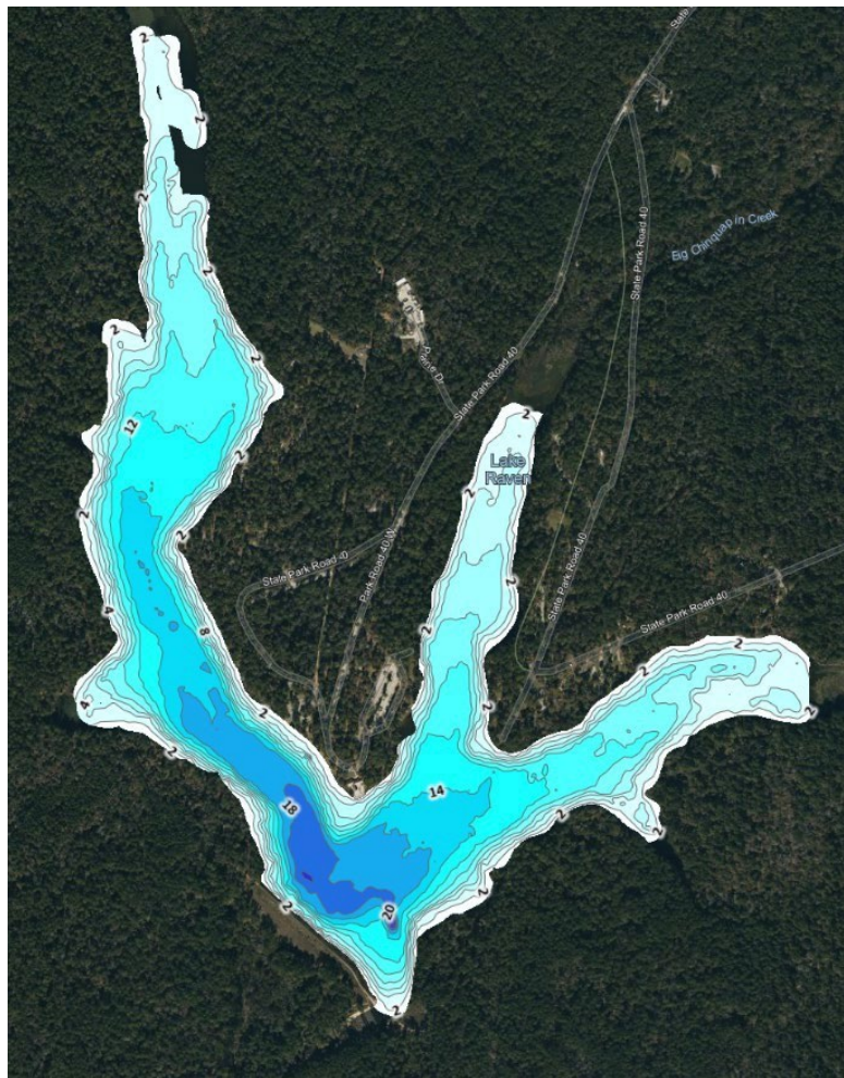
Figure 1. Bathymetric map of Lake Raven, Texas 2021. Data was collected using side scan and rendered using BioBase© software.
