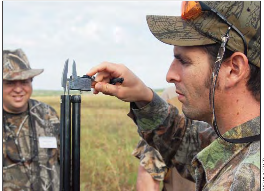
Matt Symmank gauges the choke diameter of a shotgun, while Mark Klym looks on.
