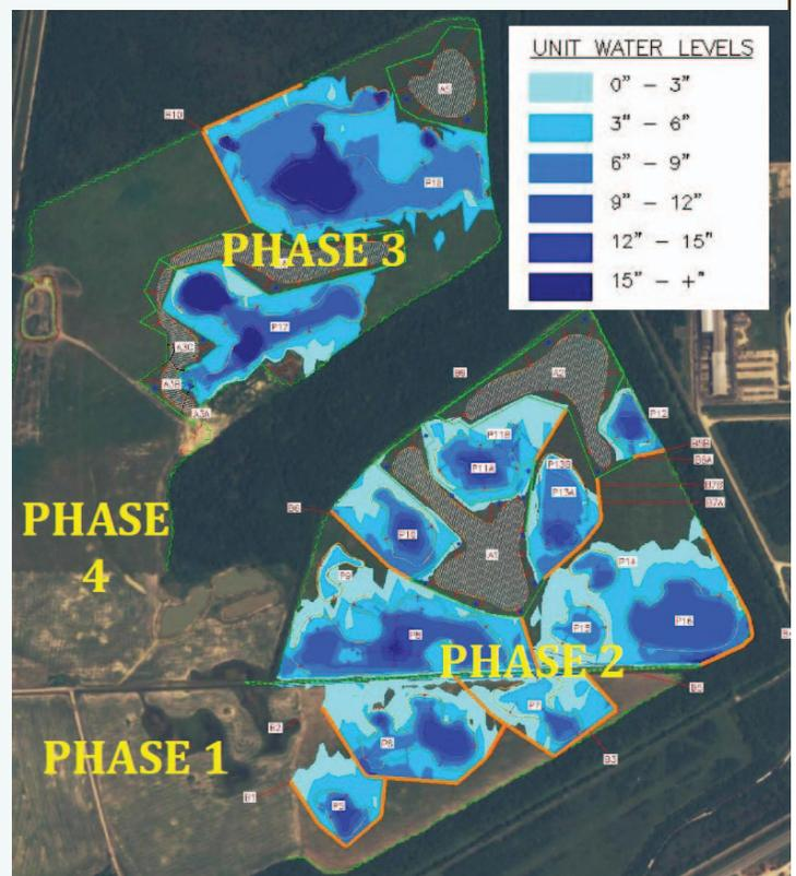
Figure 3. Close-up of the excavation and berm boundaries for Pond 6, Phase 2.
