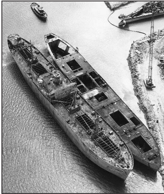
Aerial view of two of the twelve Liberty Ships being prepared for sinking as artificial fishing reefs by the Texas Coastal and Marine Council. The ship on the right has had the superstructure and main deck removed. Deck openings seen here plus large side windows provided water circulation and access for fish. Work was done under contract by Andy International, Incorporated of Brownsville, Texas.
