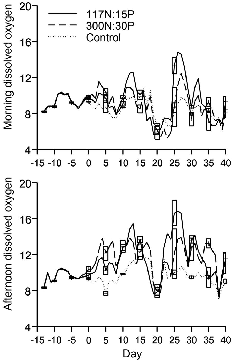
Figure 3.—Trends of morning and afternoon dissolved oxygen (mg/L) in ponds fertilized with cottonseed meal only (Control), cottonseed meal plus 300  $\mu\text{g}$  N/L and 30  $\mu\text{g}$  P/L three times weekly (300N:30P), or cottonseed meal plus 117  $\mu\text{g}$  N/L and 15  $\mu\text{g}$  P/L three times weekly (117N:15P) at the Dundee state fish hatchery in spring 2007. Boxes are standard errors at 5-d intervals for clarity.
