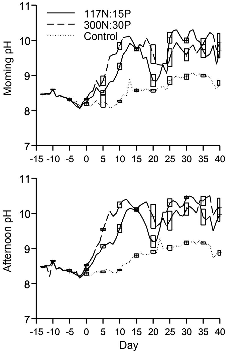
Figure 2.—Trends of morning and afternoon pH in ponds fertilized with cottonseed meal only (Control), cottonseed meal plus 300  $\mu\text{g}$  N/L and 30  $\mu\text{g}$  P/L three times weekly (300N:30P), or cottonseed meal plus 117  $\mu\text{g}$  N/L and 15  $\mu\text{g}$  P/L three times weekly (117N:15P) at the Dundee state fish hatchery in spring 2007. Boxes are standard errors at 5-d intervals for clarity.
