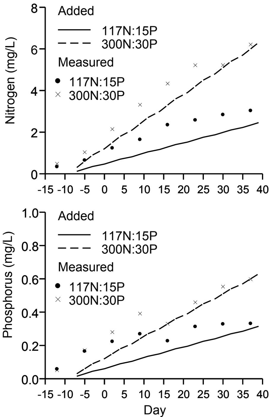
Figure 7.—Relationship between inorganic nitrogen or phosphorus added as fertilizer and concentrations measured in ponds fertilized with cottonseed meal plus 300  $\mu\text{g}$  N/L and 30  $\mu\text{g}$  P/L three times weekly (300N:30P) or cottonseed meal plus 117  $\mu\text{g}$  N/L and 15  $\mu\text{g}$  P/L three times weekly (117N:15P) at the Dundee state fish hatchery in spring 2007.
