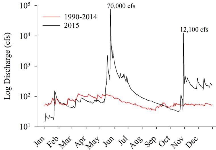
FIGURE 2.— Discharge (24-year median of daily means) from the Blanco River at Wimberley, Texas (USGS gage: 8171000) from years 1990 to 2014. Overlaid is the mean discharge for year 2015 with peak values during the catastrophic flood even in the months of May and October.
