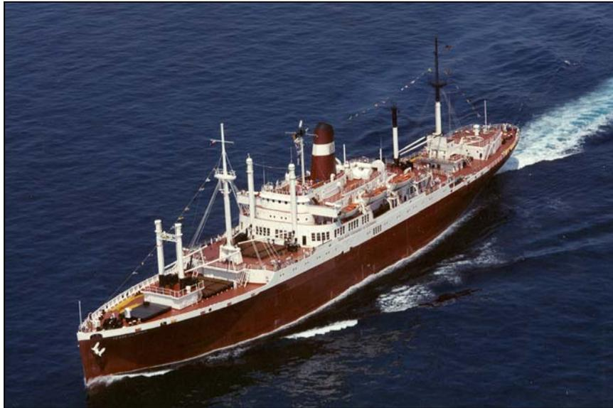
Figure 4. USTS *Texas Clipper* era from 1965-1996. Alterations made during service at Texas Maritime Academy: Crow's nest removed. No. 1 hatch cargo booms removed. Foremast booms removed. Aftermast booms removed. Swimming pool removed. Wooden decks removed. Chain telegraphs replaced. Awning rails removed. Wooden doors on P-deck removed.
