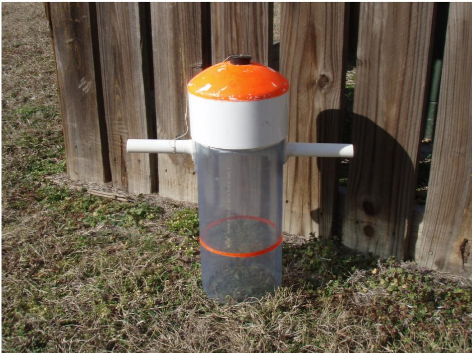
**Figure 10. 15 cm PVC corer with cap.**
