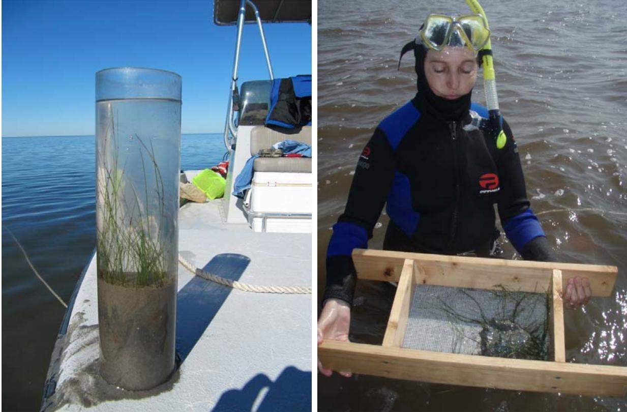
Figure 11. Left - A 9 cm corer used to collect *Halodule* and *Syringodium* samples.
