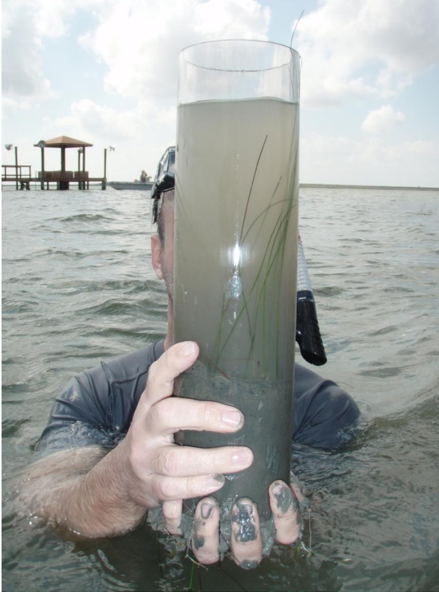
Figure 15. Seagrass corer (9 cm inner diameter) used for sampling *Halodule*, *Syringodium*, *Ruppia* and *Halophila*.
