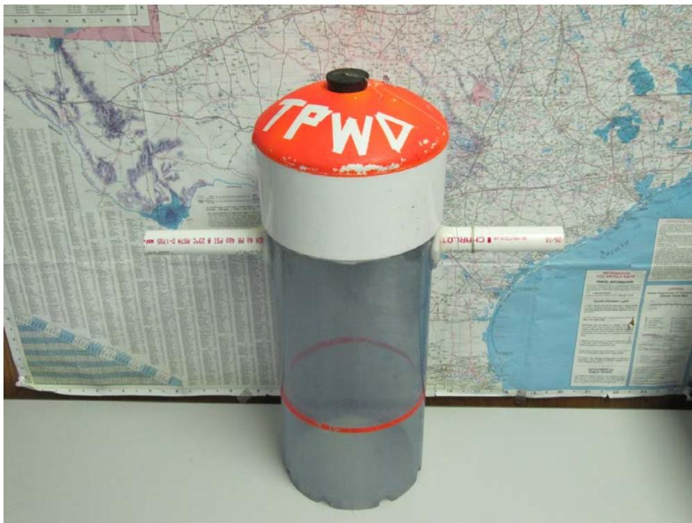
Figure 14. Seagrass corer (15 cm inner diameter) used for sampling *Thalassia*.
