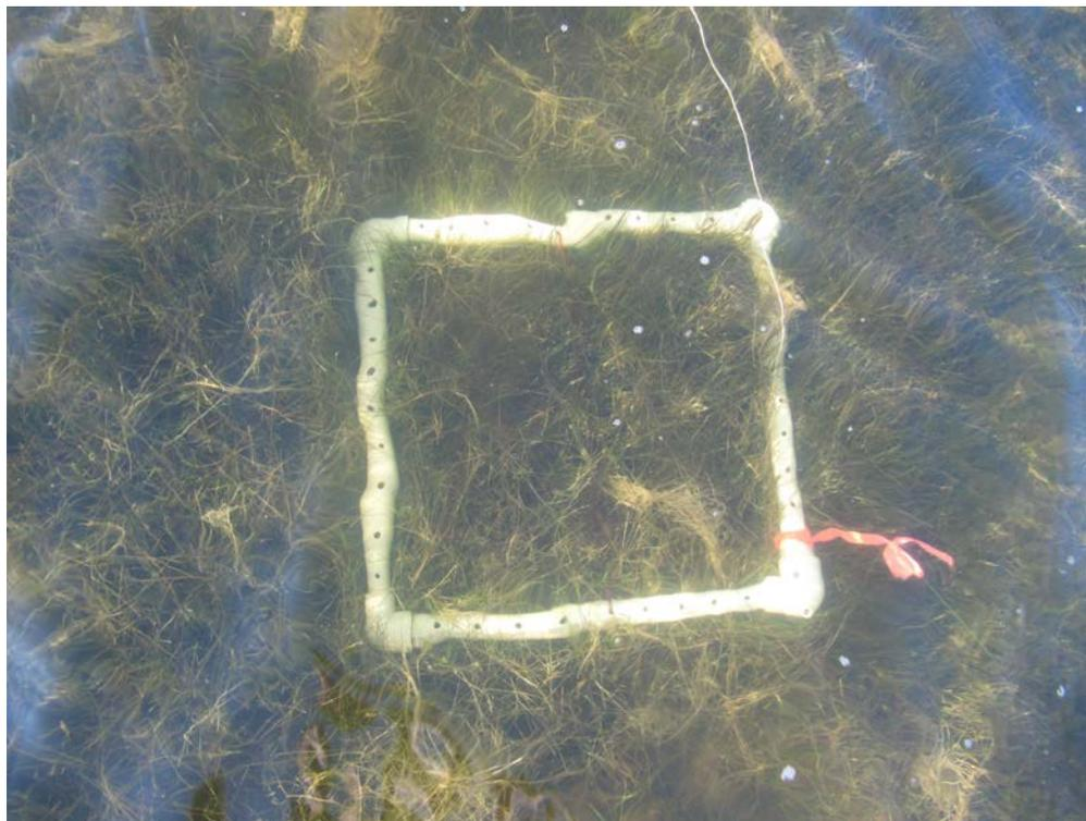
**Figure 13. Quadrat for determination of seagrass percent coverage by species. Quadrat is 0.50 m by 0.50 m (0.25 m<sup>2</sup>) and constructed of white PVC.**
